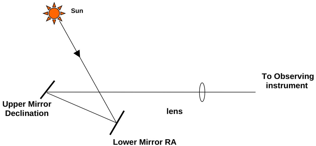
**Figure – 1 Coelostat mirror arrangement**
