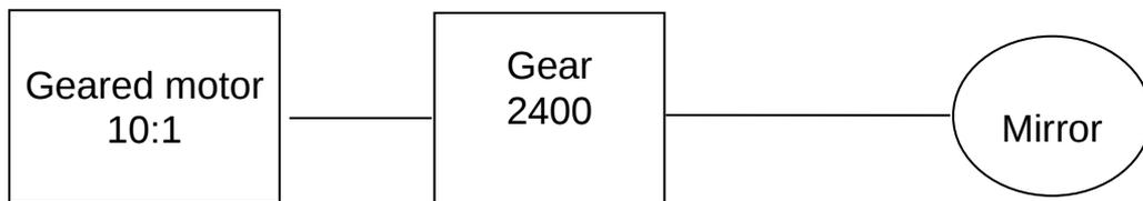
**Figure – 2 Track Axis Gear Ratio**
