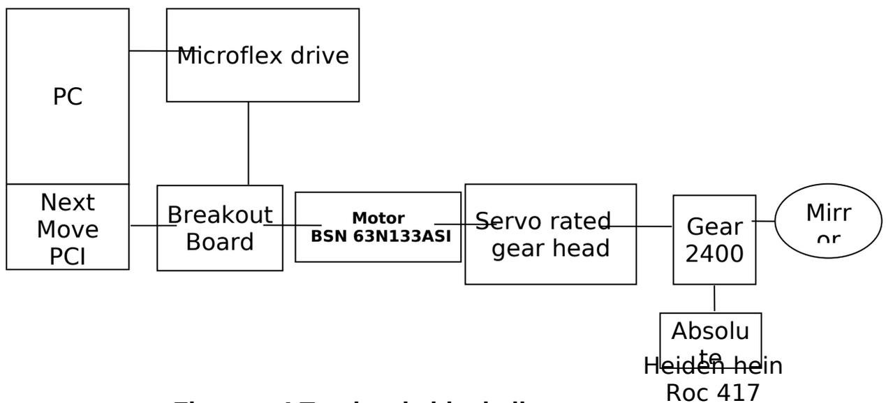
**Figure – 4 Track axis block diagram**
