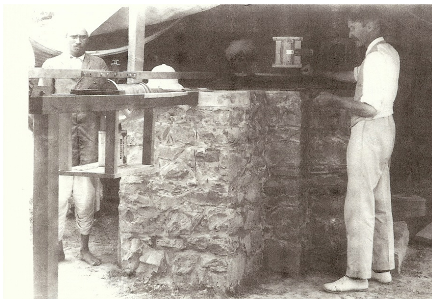
Fig. 2. John Evershed working with the spectroheliograph at the Kodaikanal Observatory (from IIA archives)
