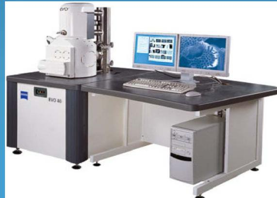
Scanning Electron Microscope EVO 40, Carl Zeiss
