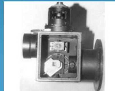
Rotational Shearing Interferometer
