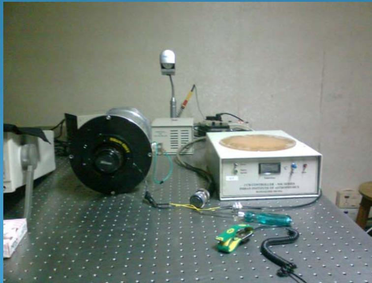
Lab setup for acquiring an image using CCD DEWAR.
