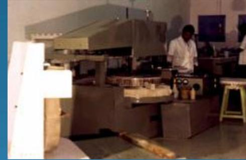
The picture shows 30 inch & 18 inch polishing machines. The primary mirror of the 30 inch telescope optics were fabricated using these machines during 1980s.
