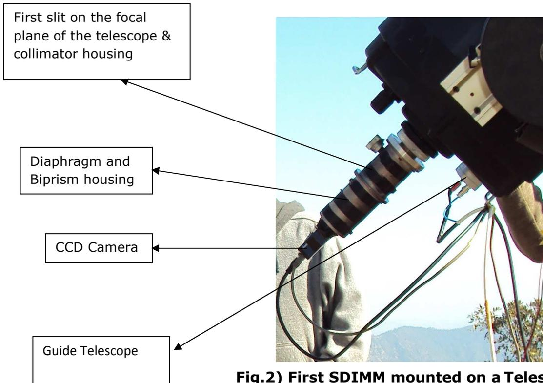
**Fig.2) First SDIMM mounted on a Telescope**
