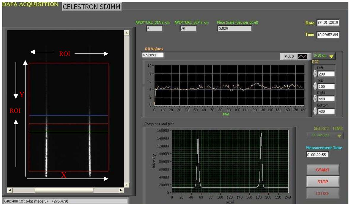
**Fig 3.) Front panel for Data Acquisition (LabVIEW Platform)**
