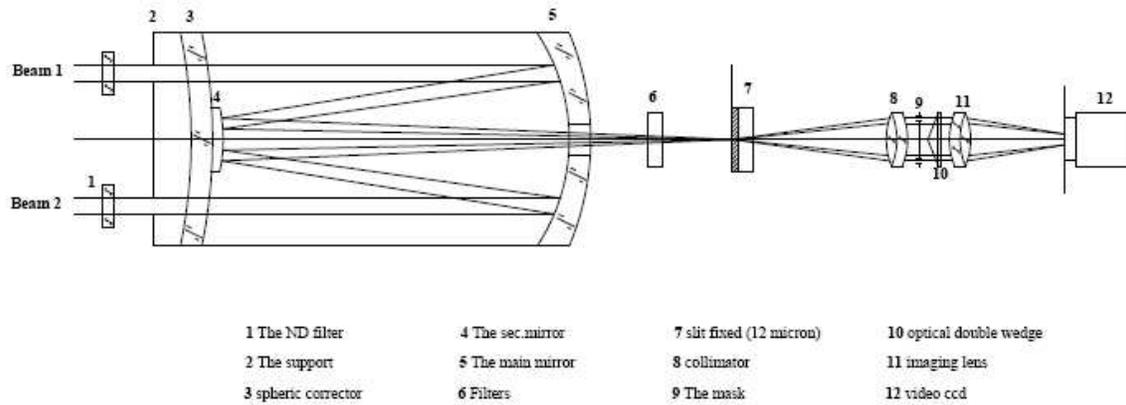
**Fig.1) Optical setup of SDIMM**
