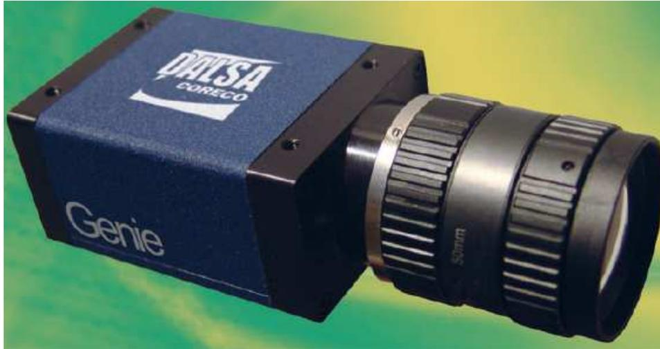
The Genie M640 with a resolution of 640 x 480 CCD has been used. Operating at 60 frames per second at full resolution, the Genie M640 takes advantage of gigabit Ethernet technology for transmitting data and direct link from the camera to a PC. All Genie cameras are supported by DALSA's Sopera™ LT software libraries featuring CamExpert for simplified camera set-up and configuration.
