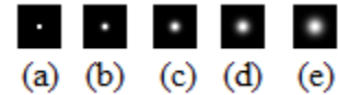
Figure 2 Gaussian spots with a spread, \sigma taking values (a) 0.5 (b) 1.0 (c) 1.5 (d) 2.0 (e) 2.5 (image center is the spot center)
