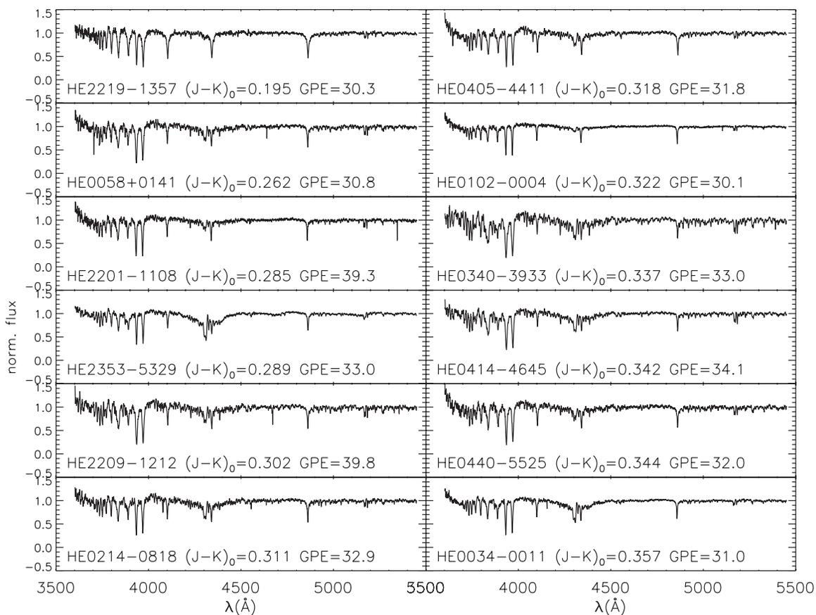
Figure 6. Example of CEMP candidates observed based on the new line index criteria. The spectra were taken with Goodman spectrograph on the SOAR telescope.
