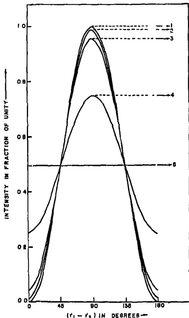
Fig 3 Fringe profile for different errors in axes
