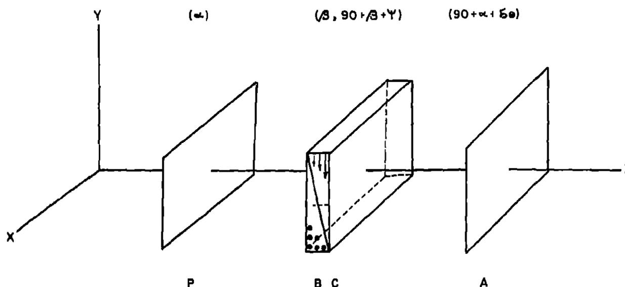
Fig 1 Schematic arrangement of Babinet Compensator
