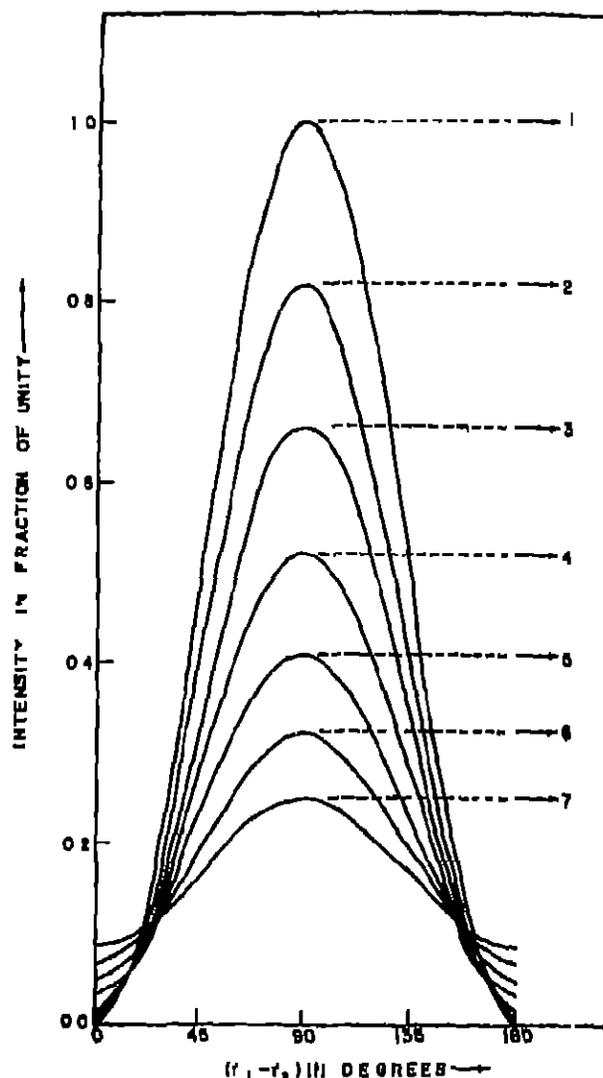
Fig. 2. Fringe profiles for different degrees of imperfection of the polaroids. 1. Perfect polaroids, 2 to 7. Imperfection  $B_{11}$  to  $30\%$ .
