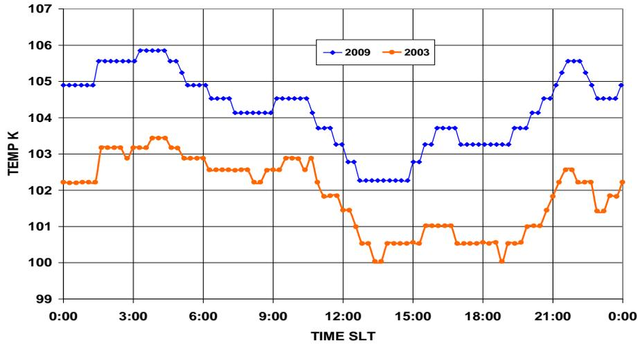
**Figure : 7a** KALPANA-1 VHRR Radiant Cooler Patch Temperature during Summer Solstice
