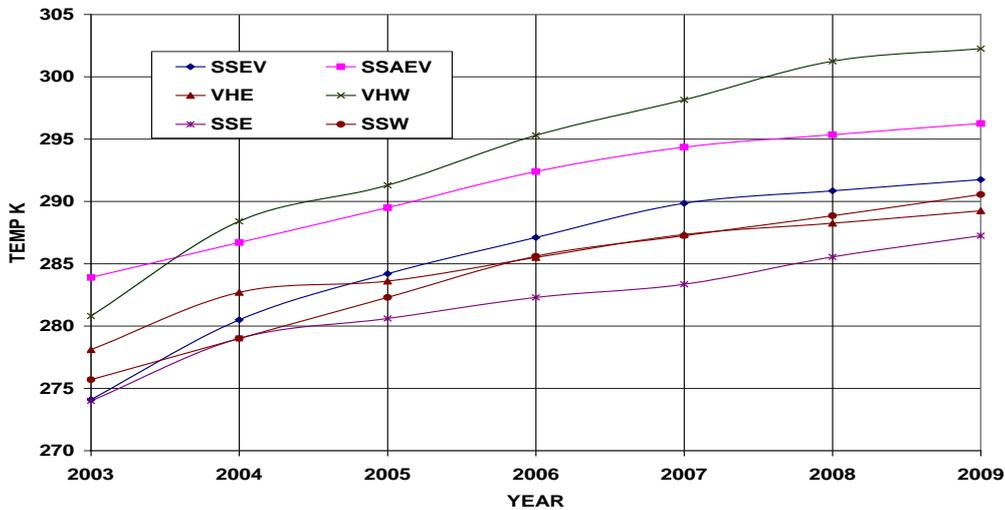
**Figure : 8c** KALPANA-1 VHRR Radiant Cooler Temperature (Max) Variation over Years during Summer Solstice
