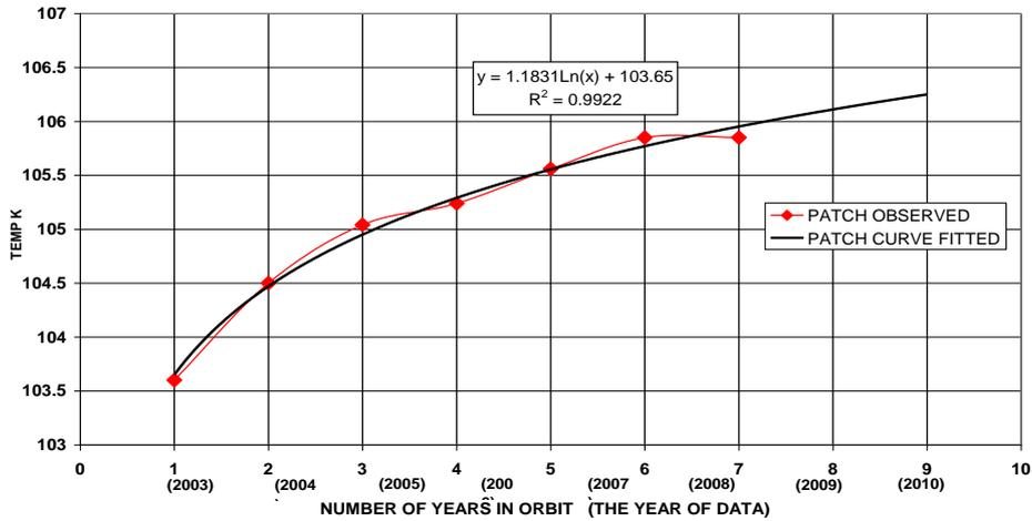
**Figure : 7b** KALPANA-1 VHRR Radiant Cooler Patch Temperature (Max) variation over years during Summer Solstice
