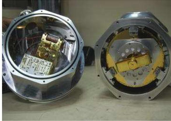
Figure 1: Left panel: Preamplifier board is mounted which will be coordinating output signal of CCD to its controller that is connected to a PC; Right panel: CCD Dewar is filled with LN<sub>2</sub> (Liquid Nitrogen) to cool the CCD.
