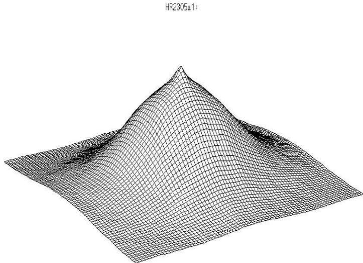
Figure 1: Autocorrelation of seeing disk, as well as of speckle component.
