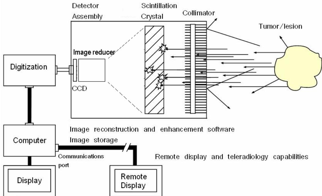
Fig. 1 Schematic of a Gamma camera
