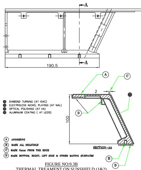
The process developed for INSAT 3D sun shield panels is as follows:
