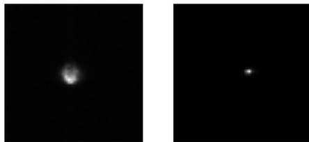
*Fig. 9.13 Image captured by Andor CCD camera with 10 msec exposure time. Left: uncorrected image. Right: Corrected image (Twice magnified)*
