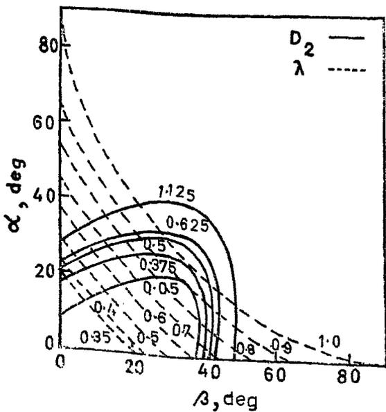
Fig. 5— $D_2(\alpha, \beta)$  (—) and  $\lambda(\alpha, \beta)$  (---) against  $\beta$  for different values of incidence  $\alpha$
