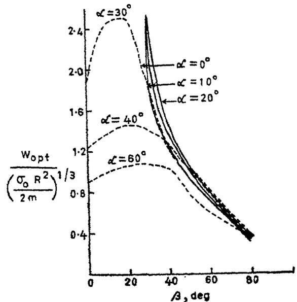
Fig. 11—Variation of  $w_{opt}/(\sigma_0 R^2/2m)^{1/3}$  with  $\beta$  at different values of angle of incidence  $\alpha$
