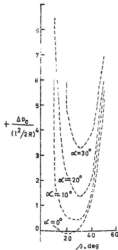
Fig. 7—Variation of  $\Delta p_c / (l^2 / 2R)$  with  $\beta$  at different values of angle of incidence  $\alpha$
