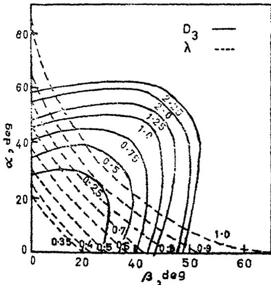
Fig. 9— $D_3(\alpha, \beta)$  (—) and  $\lambda(\alpha, \beta)$  (---) against for different values of angle of incidence  $\alpha$
