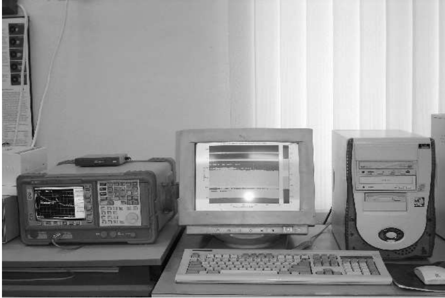
Figure 3. Gauribidanur Radio Array Solar Spectrograph (GRASS). The agilent spectrum analyzer along with control and data acquisition PC are shown.
