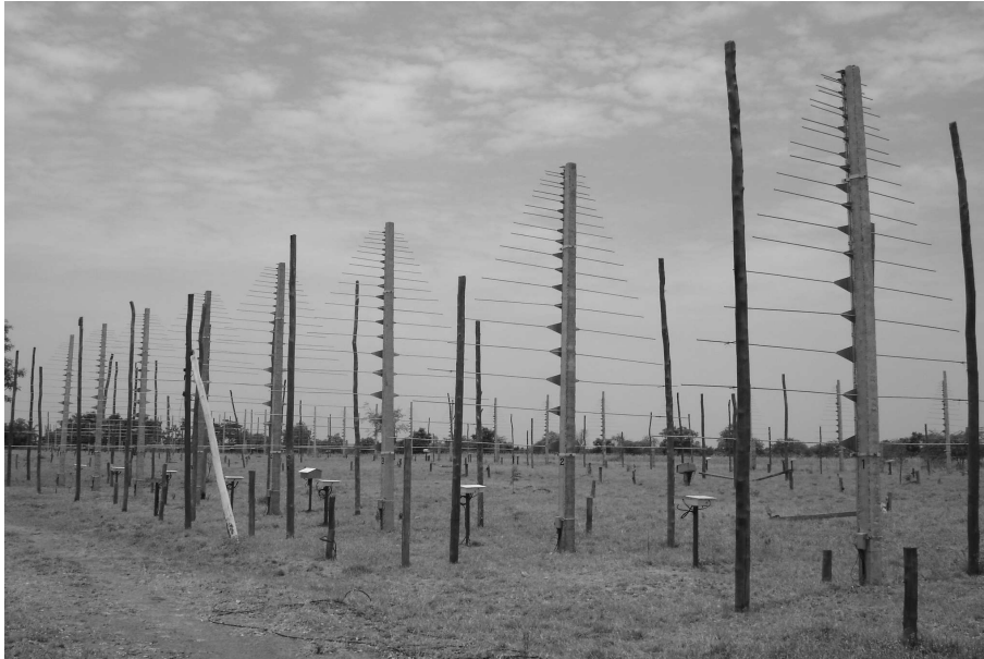
Figure 1. Antenna system for the GRASS. Eight log periodic dipoles stacked along the north - south direction with their E -plane along the east-west direction are shown. The inter-element spacing is 7 m along the north - south direction.
