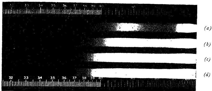
Fig. 3 Transmission limits of amethyst quartz in the ultraviolet, (specimen A 1 ), for different exposure times (a) 1 minute, (b) 3 minutes, (c) 7 minutes, (d) 15 minutes
