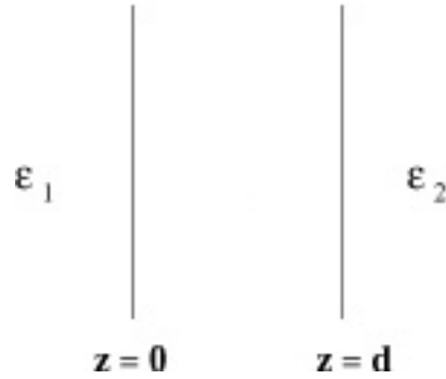
Fig. 1.2: Two semi-infinite dielectric slabs of dielectric constants \epsilon_1 and \epsilon_2 , placed distance d apart in vacuum.
