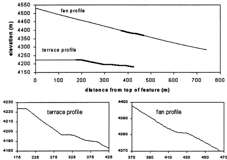
Fig. 4. Profiles across the fan and the terraces. Small insets show details of the three fluvial terraces and of the fault with its 5 m of reverse faulting. These correspond to the heavy lines in the larger plot.
