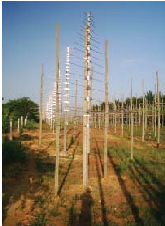
A close up view of 135^{\circ} and 45^{\circ} oriented antennas
