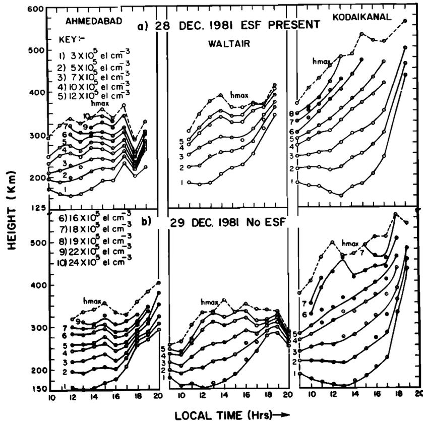
Fig. 2. Height variation of constant electron density contours (solid lines) and  $h_m F_2$  (dashed lines) during daytime at the three stations on (a) ESF and (b) no-ESF days.
