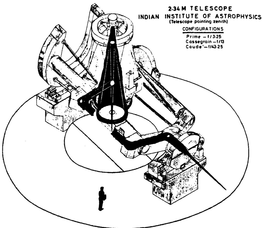
Fig. 6—Sketch of the proposed optical system
