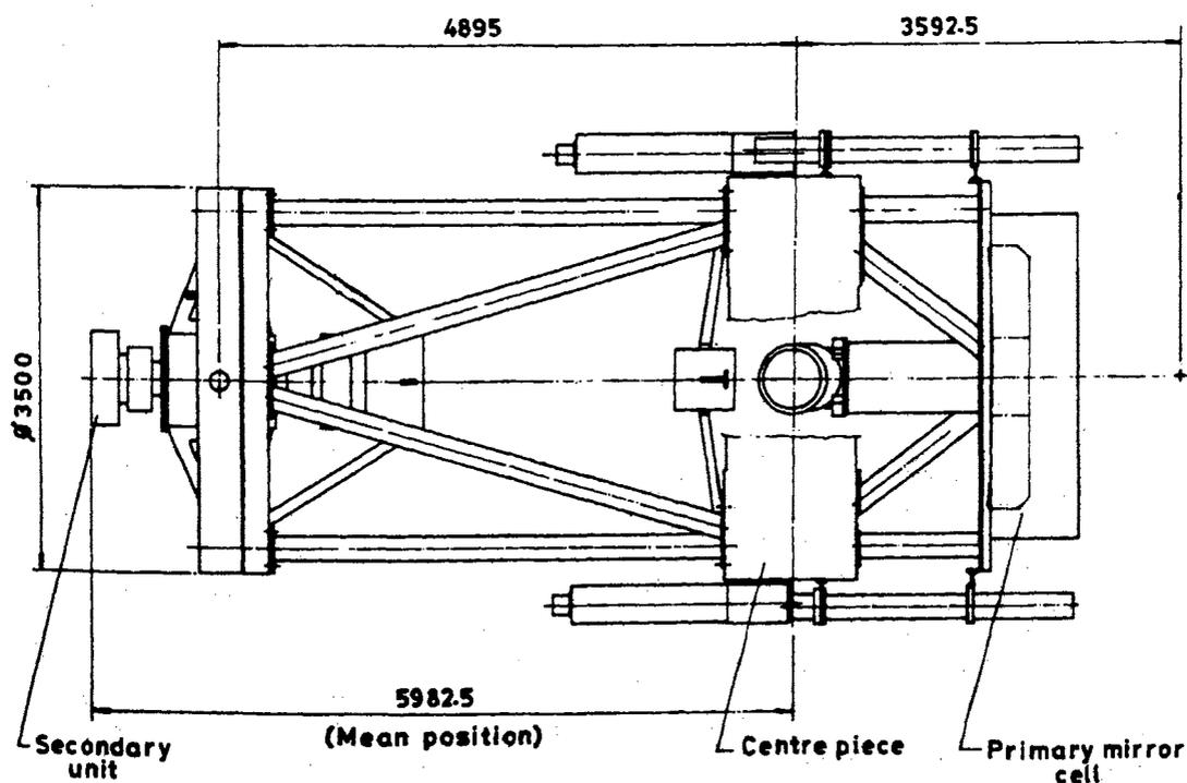
Fig. 2—Serrurier truss of 234 cm telescope
