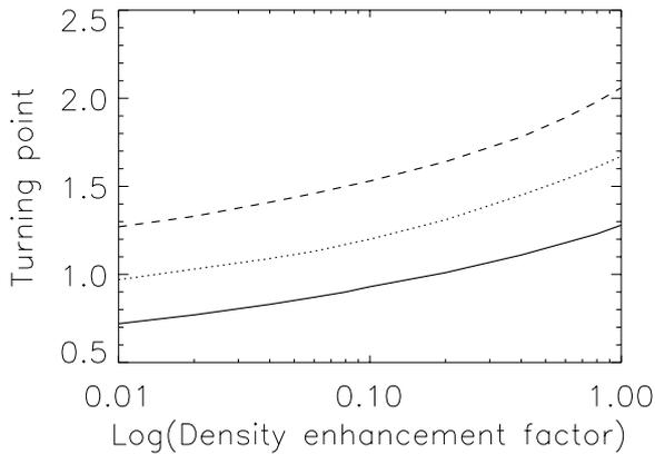
**Fig. 4.** Variation of turning point in solar radii at 34.5 MHz with the density enhancement factor. The solid curve is for density gradient 3.32 and the dotted one for 4.32 and the dashed one for 5.32.
