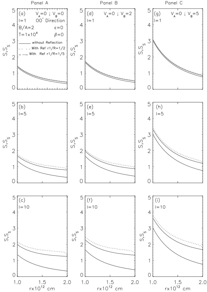
**Figure 3.** Source functions  $S$  and  $S_s$  (which are normalized to intensity units) with respect to radius in a scattering medium for shown parameters in panel A. Panel B is same as panel A but  $V_A = 0$  and  $V_B = 2$  mtu. Panel C is same as panel B but  $V_A = 0$  and  $V_B = 5$  mtu.
