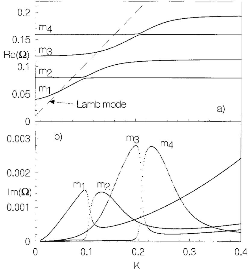
Figure 1. Part of the diagnostic diagram showing the interaction between the magnetic modes with Lamb mode, for a dimensionless radiative relaxation time  $\bar{\tau}_R = 0.05$ . Variation with  $K$  of the (a) real (solid lines) and (b) imaginary (dotted lines) parts of the frequency. In panel (a) the dashed line marks the location of the adiabatic Lamb mode.
