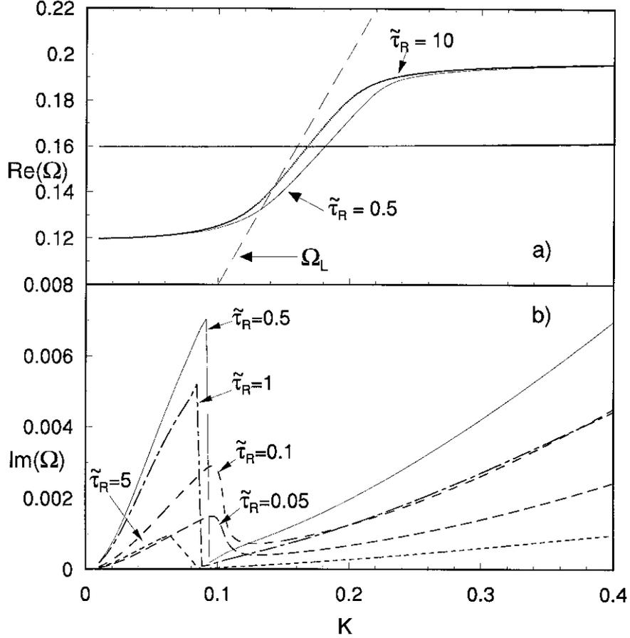
Figure 2. Region of interaction between  $m$ - and Lamb-type solutions for different values of  $\tilde{\tau}_R$  as labeled. Variation of (a) real part and (b) imaginary part of the frequencies with  $K$ . The dashed line in (a) shows the adiabatic Lamb mode.
