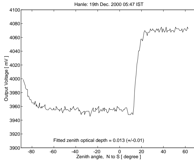
Figure 4. A typical averaged scan, detected voltage as a function of zenith angle. The trace from zenith angle between 15^\circ and 22^\circ is the transition voltage as the mirror begins to partially look at sky and the absorber. The higher voltage between 22^\circ and 60^\circ is the reference voltage when the mirror fully looks at the absorber.
