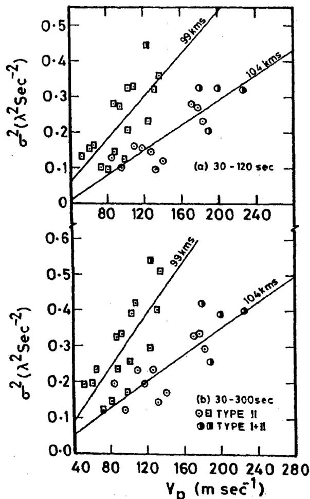
Fig. 4. Plots showing the dependence of the variance ( $\sigma^2$ ) of 30-300 s and 30-120 s fluctuations in  $\dot{P}$  at Kodaikanal on the phase velocity ( $V_p$ ) of electrojet irregularities at 99 (squares with dots) and 104 km (circles with dots) measured with VHF coherent backscatter radar Thumba. The nature of the Doppler power spectrum (type II/combination of type I and II) from which  $V_p$  is deduced is also indicated.
