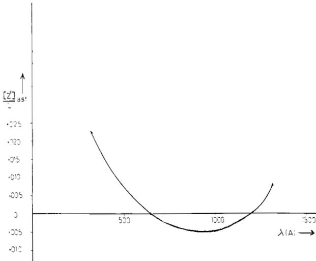
FIG 3. — Astigmatism per unit grooves length at different wavelengths.
