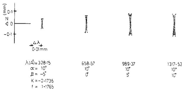
FIG 5. — Spot diagrams at different wavelengths.
