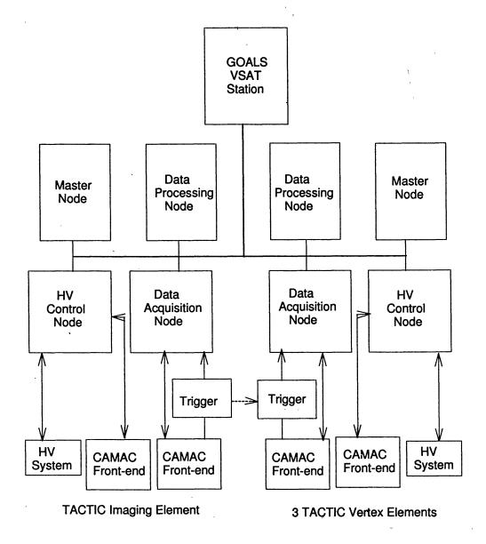
**Figure 1.** Block diagram of the multinode data acquisition and control system of the 4-element TACTIC telescope array.
