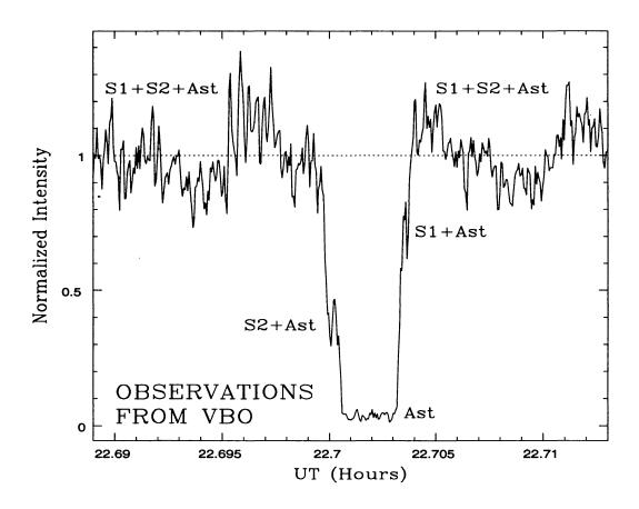
Figure 1. Light curve recorded at the 102 cm telescope at VBO. The normalized flux level outside the event, S1, S2, and Ast corresponds to contributions from the components A and B of the star and the asteroid respectively. The brighter component A was occulted first and about 2.8 seconds later, the fainter component B went behind the asteroid. The stars made the reappearance in the same order.
