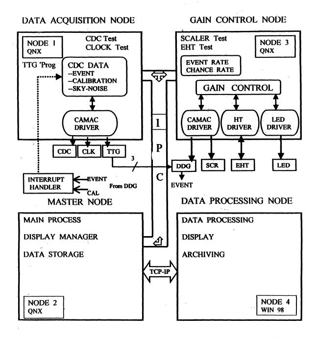
Figure 1. Block diagram representation of the multi-node Vertex Element Data Acquisition System (VEDAS) of the TACTIC telescope array.
