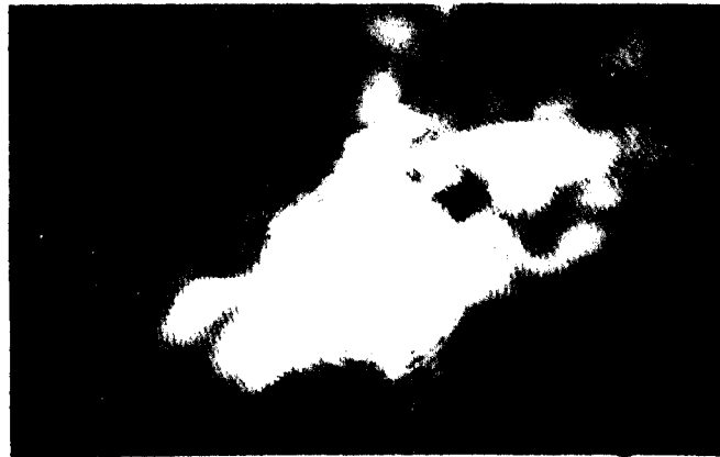
- Cross section of a laser beam after propagation through a 800 m path.
