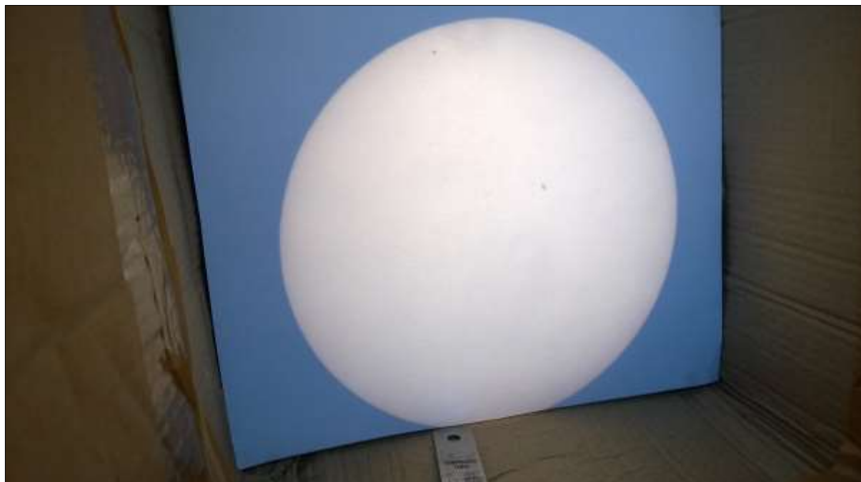
Figure 31: The 9 May 2016 transit of Mercury, with observed with a tripod-mounted 89/1400 mm Questar at the author's residence in Bengaluru. The ~9-inch diameter solar image shown here at 17:09 IST was projected onto a white board inside a carton that was fastened to a wall. Mercury is the small dot just left of top centre (photograph: R.C. Kapoor).
