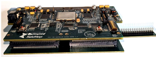
Figure 6.1: Fabricated DMD Chipset FPGA board with dual FMC interface board.
