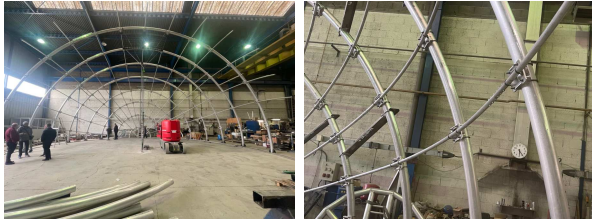
Figure 5.11: Left: A portion of main frame which will support LED panels; Right: A close-up of the same, assembled at vendor location in France.
