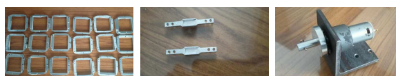
Figure 6.18: Aluminium filter cells, filter clamping pad, and gasket for IFS filter wheel.
