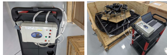
Figure 6.4: Left: SSA Test Controller developed at IIA; Right: Undergoing functionality testing at ITOFF.
