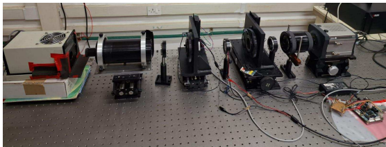
Figure 6.10: Lab setup for full Stokes polarimeter for characterisation of retarder.
