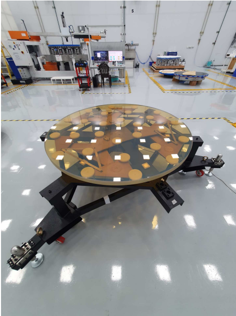
Figure 5.1: First TMT polished roundel churned out from ITOFF, IIA.
