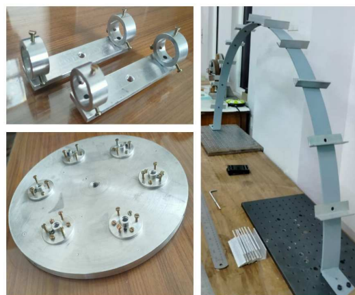
Figure 6.19: (left) Laser holder, (bottom) Nasmyth telescope concept, (right) Laser holder arch
