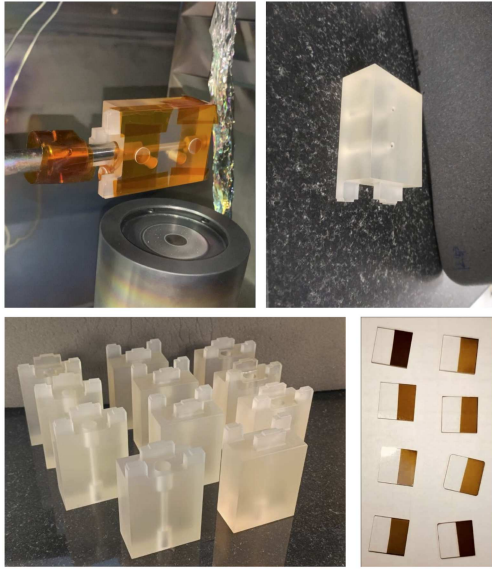
Figure 6.3: Clockwise from top left: 8 coupons on TMT Edge Sensor block; Chromium coated coupons; ultrasonic machining at Optica; 15 machines blocks.
