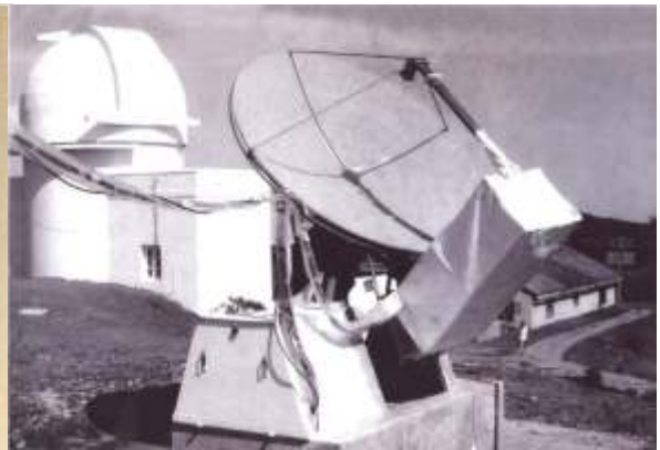
The 3 GHz antenna system in front of the KTT.
