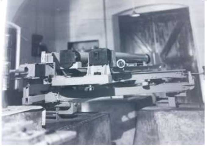
A picture of siderostat light feeding system with mechanical tracking. A Spectroheliograph capable of making Ca-K and H-alpha image of the sun.
