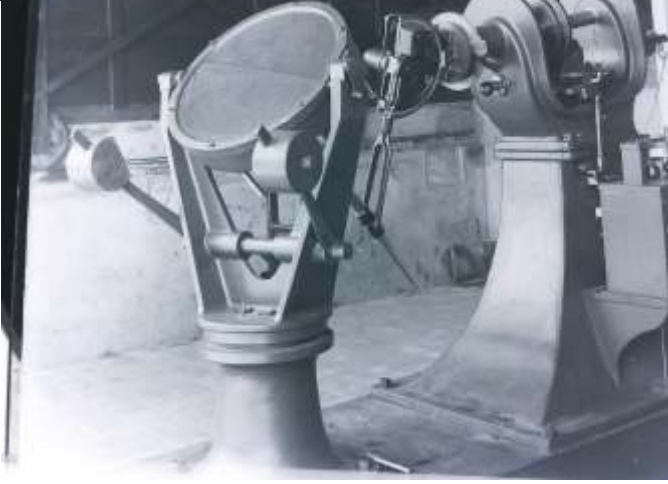
A picture of siderostat light feeding system with mechanical tracking. A Spectroheliograph capable of making Ca-K and H-alpha image of the sun.
