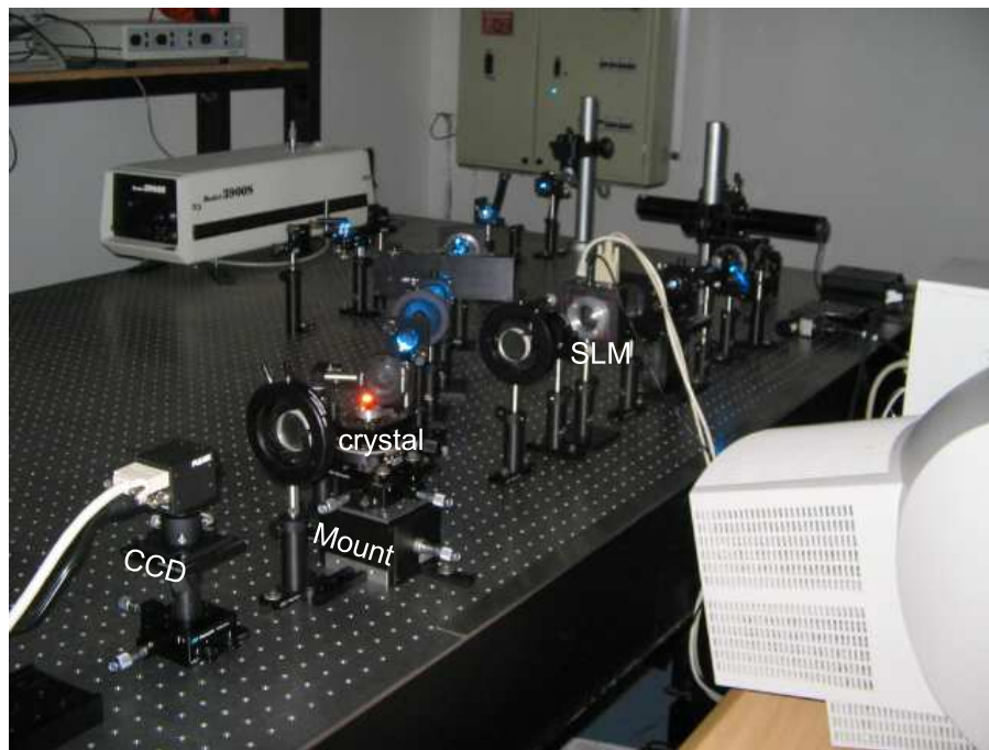
Figure 4.9: A photograph of holographic data storage and retrieval system in the lab.
