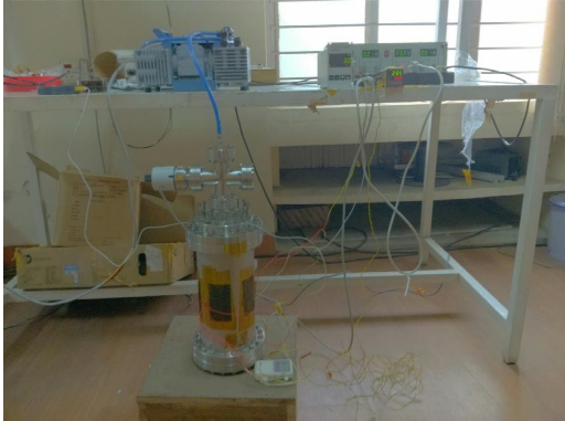
Figure 4.4: Precision thermal control vacuum chamber ( 0.01^{\circ} C thermal stability)
