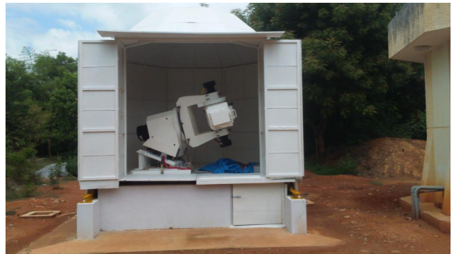
Figure 4.3: H-alpha Telescope housed inside the sliding enclosure at CREST, Hosakote.
