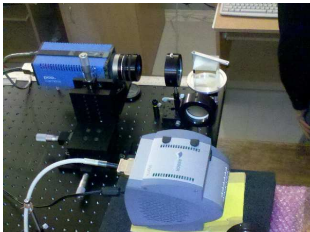
Dual channel imaging system at WARM telescope. PCO2000 and ANDOR iXON 888 model CCDs are used to image the Sun in G-band (pass band=8Å) and narrow band (pass band = 4.5 Å) red filter respectively.
