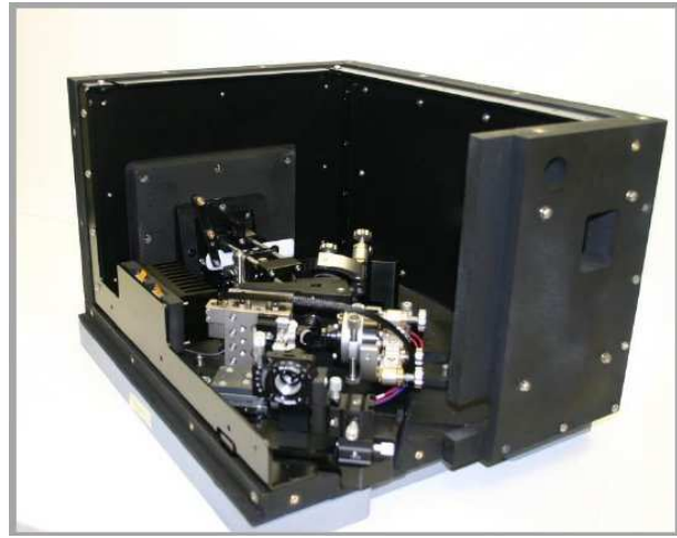
The cassegrain unit of the High Resolution Spectrograph for HCT. It comprises of fold mirror, pinhole mirror, input selector and guide camera. The right figure shows the complete unit with its thermal enclosure.
