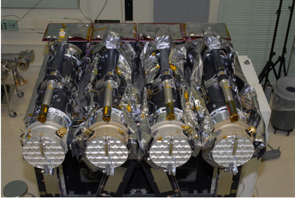
FIGURE 2.4: The four AIA telescopes mounted on the SDO spacecraft during integration at NASA's Goddard Space Flight Centre. Image credit: Lemen et al. (2012)
