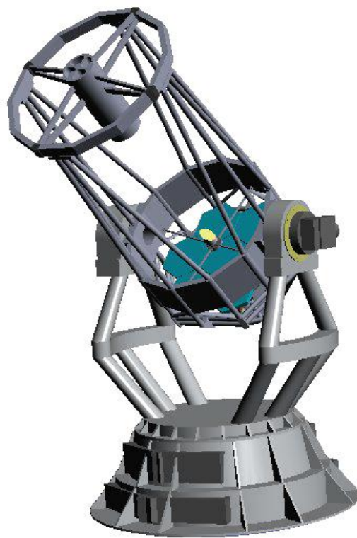
Figure 1-6. A conceptual view of the Prototype Segmented Mirror Telescope (PSMT). PSMT is a seven segment telescope with a primary mirror of 1.5m in diameter.
