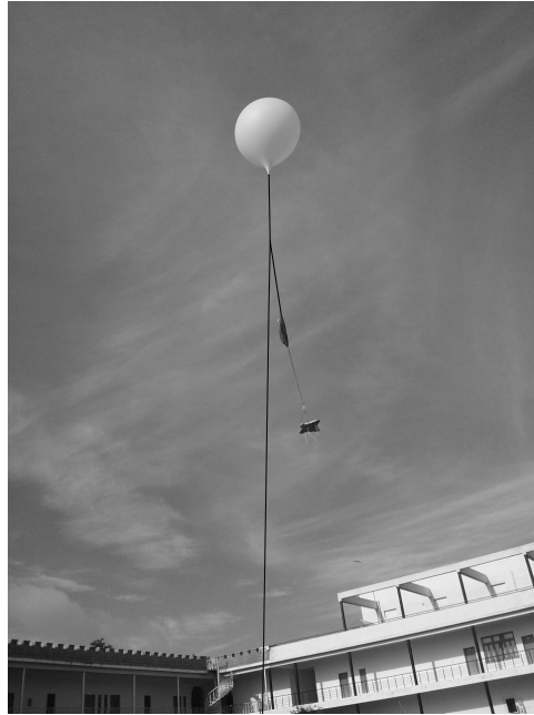
Figure 6.19: The star-shaped platform is connected to the balloon through a parachute. The entire system is tethered to a spindle on the ground (not shown in figure) using a nylon tether of approximately 200 m length.
