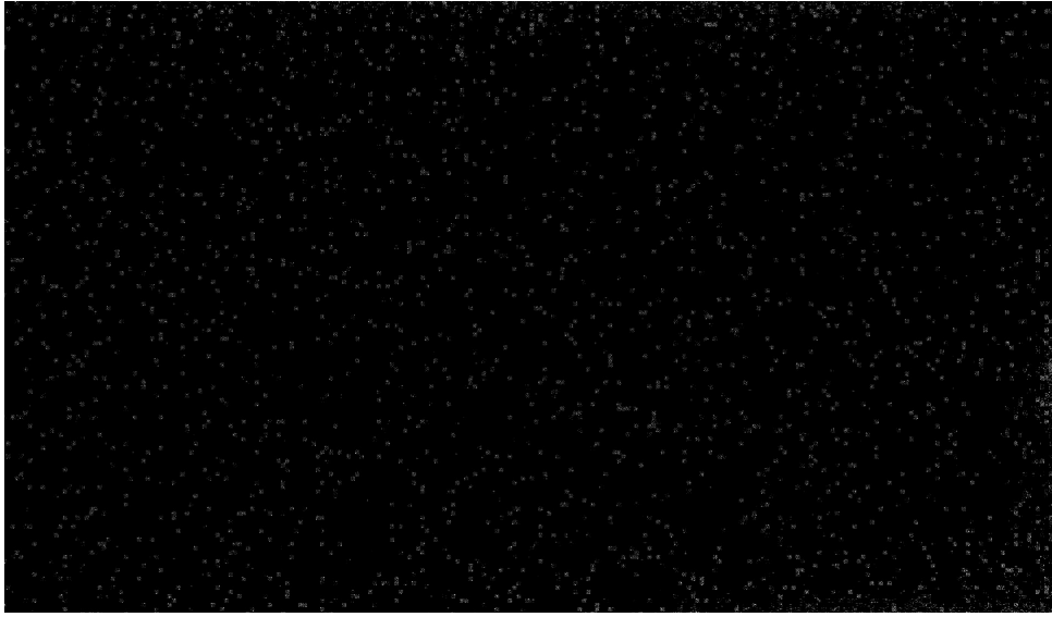
Figure 5.7: (Top:) A dark frame generated from our image sensor by giving an exposure of 12s in log scale. The hot pixels are visible in the image.
