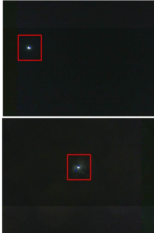
Figure 6.10: Top: One of the images taken during the ground test when the magnetometer was not calibrated. Bottom: The image of the Moon taken during the ground test where the magnetometer is calibrated for hard iron and soft iron biases. The position of the Moon is marked in a rectangle.
