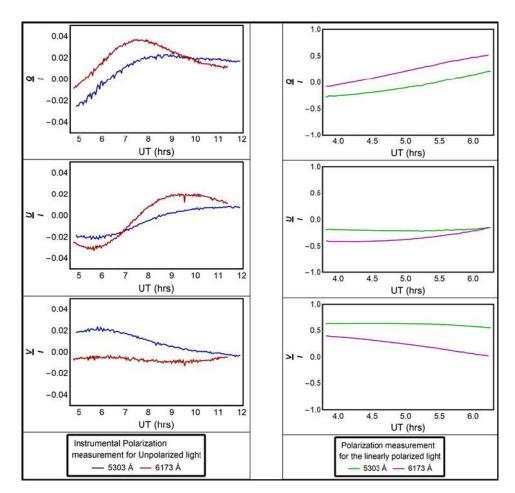
Figure 7.17: The instrumental polarization and linear polarization measured at the telescope focus at  $\lambda = 5303$  Å and 6173 Å
