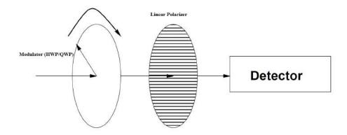
Figure 1.3: A simple polarimeter with a rotating modulator and a fixed linear polarizer (Keller, 2002)
