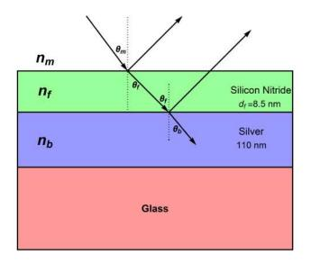
Figure 4.5: The coating used in the analytical modeling for TMT. Silver is the bulk metal layer. Silicon Nitride is the protective layer.
