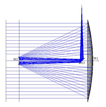
Figure 6.2: Optical layout of TMT with segmented primary mirror obtained from  $Zemax^{(R)}$ .
