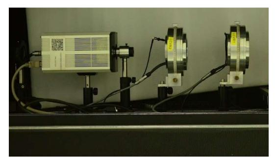
Figure 7.4: Imaging spectropolarimeter at the MAST telescope
