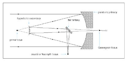
Figure 1.5: Schematic of a Cassegrain telescope showing the use of a flat tertiary mirror to direct the light toward Nasmyth or Coudé focus.
