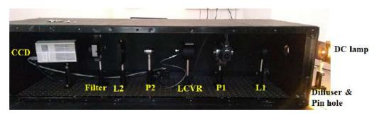
Figure 7.13: Experimental setup for the characterization of LCVR. L1 and L2 correspond to the collimating and imaging lens respectively. P1 and P2 are the Glan Thompson Polarizing Prisms with extinction ratio of  $10^{-6}$
