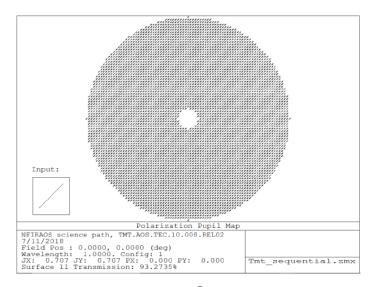
Figure 3.2: Polarization pupil map in Zemax<sup>®</sup> at the Nasmyth focus of the Thirty Meter Telescope (TMT) for linearly polarized light at  $45^{\circ}$  as the input. The grid has  $83 \times 83$  rays across the pupil.
