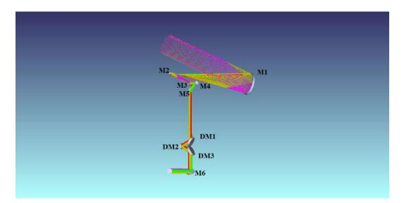
Figure 7.2: Optical layout of the Multi-Application Solar Telescope obtained from Zemax<sup>®</sup>
