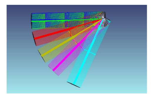
Figure 4.28: The optical layout form  $Zemax^{(R)}$  showing different zenith angles of the telescope
