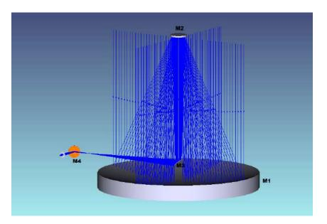
Figure 4.22: Mirror (M4) on the Nasmyth platform for cancellation of polarization effects
