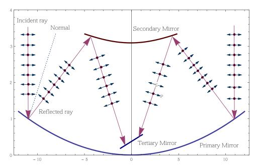
Figure 4.3: The TMT representation showing ray diagram and mirrors.
