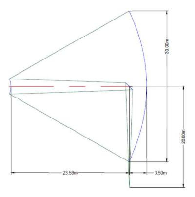
Figure 4.1: Optical Layout of the Thirty Meter Telescope showing the folded Ritchey-Chretien layout (TMTGroup, 2012).
