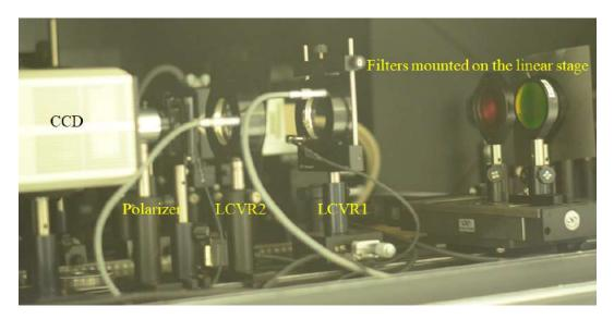
Figure 7.15: The polarimeter placed at the telescope focus after the M6 mirror
