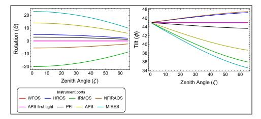
Figure 4.27: The rotation and tilt of the Nasmyth mirror (M3) at all the instrument ports.
