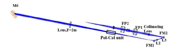
Figure 7.3: The components in the optical path between M6 mirror and imaging spectropolarimeter at MAST obtained from  $\text{Zemax}^{\textcircled{R}}$
