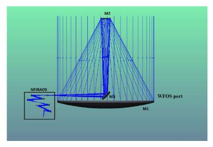
Figure 5.1: Optical Layout of the Thirty Meter Telescope with WFOS port and NFIRAOS instrument. The Nasmyth mirror has  $\Phi = 45$  and  $\theta = 0$  at the WFOS port and  $\Phi = -45$  and  $\theta = 5.499$  at the NFIRAOS port.
