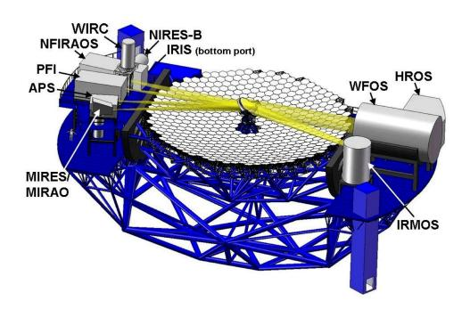
Figure 4.2: The Nasmyth platform of the TMT showing the different instrument positions. WFOS instrument port corresponds to the tilt of 45 degrees of the Nasmyth mirror (TMTGroup, 2012).
