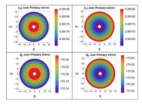
Figure 4.6: Reflection coefficients on the primary mirror surface at  $\lambda=2.583 \ \mu\text{m}$ . The top panel shows the amplitudes and the bottom panel shows the phase of the reflection coefficients.
