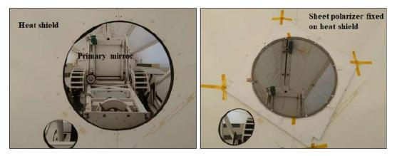
Figure 7.6: Sheet polarizer fixed on the heat shield of the telescope.
