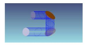
Figure 4.21: The optical layout of two inclined flat mirrors for polarization cancellation
