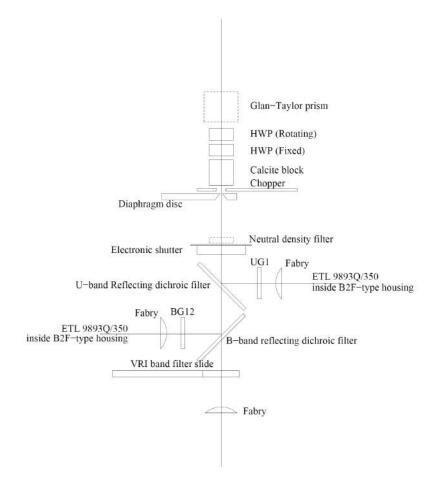
Figure 2.5: Schematic layout of the photopolarimeter showing different components at the 1 m telescope in VBO.
