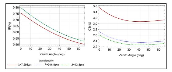
Figure 8.2: The IP and CT estimated at the modulator with varying zenith angle. The unprotected gold coating is used for the mirrors in the MICHI instrument. The values are shown at three different wavelengths in the N band.
