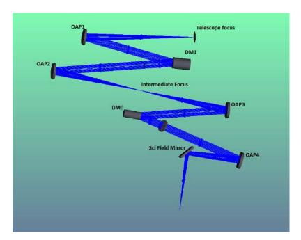
**Figure 5.12:** Optical layout of the NFIRAOS instrument for TMT. It is kept on the Nasmyth platform at an Instrument Bearing Angle (IBA)=174.5 degrees which corresponds to a tilt of -45.048 and rotation of 5.499 of the Nasmyth mirror. It consists of 4 Off Axis Parabolas(OAP), 2 Deformable Mirrors (DM) and a fold mirror.
