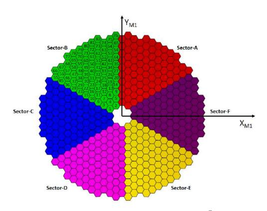
Figure 6.1: Segmented primary mirror of TMT simulated in Zemax<sup>®</sup> showing different sectors in different colours (Baffes et al., 2008). The numbering scheme of the segments is shown for Sector-B.
