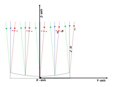
Figure 3.1: Coordinate system in the polarization ray tracing algorithm.
