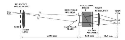
Figure 2.2: Optical layout of the imaging polarimeter at the IGO telescope (Ramaprakash et al., 1998)
