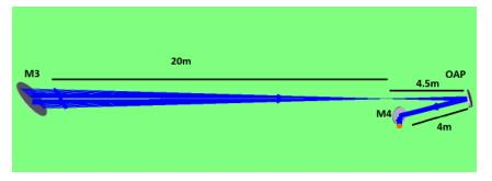
**Figure 4.23:** Mirror (M4) on the Nasmyth platform after the Off-axis parabola for cancellation of polarization effects
