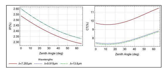
Figure 8.3: The IP and CT estimated at the focus of the imager with varying zenith angle. The unprotected gold coating is used for the mirrors in the MICHI instrument. The values are shown at three different wavelengths in the N band.
