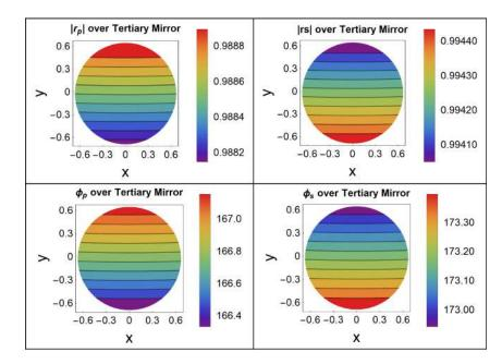
Figure 4.7: Reflection coefficients on the Nasmyth mirror surface at  $\lambda=2.583 \ \mu\text{m}$ . The top panel shows the amplitudes and the bottom panel shows the phase of the reflection coefficients.
