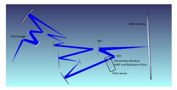
**Figure 8.1:** The optical layout of the MICHI imager obtained in  $\text{Zemax}^{\mathbb{R}}$ . The polarimetry module shows the position of the modulator and the polarizer.
