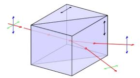
Figure 1.4: Wollaston prism showing the two orthogonal components of electric field. Image credits:Wikipedia
