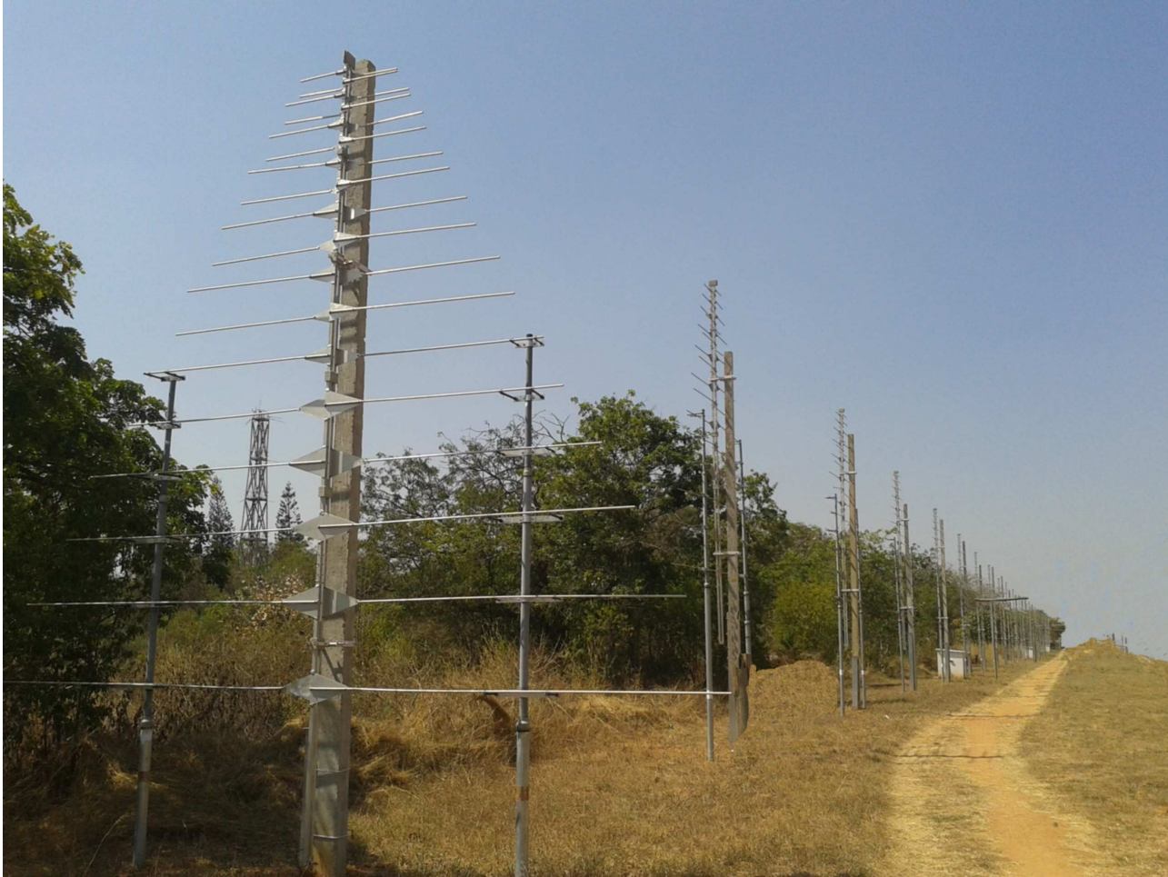
Fig. 2.9: Image shows the GRIP array. The first antenna belong to the group-2 and then onwards next 8 antennas belong to group-3. Note that in the first antenna, arms are aligned in North-South direction where as in group-3, arms of the antennas are aligned in East-West direction. From the second antenna onwards next 8 antenna belongs to group-3 and from there next 16 antennas belongs to the major group-C (group-4 + group-5). Every antenna is placed 10 meters apart from its adjacent antenna in the GRIP. The white boxes shown in the array are the group centers in which power combiners, group amplifier, DC power supply etc are kept.
