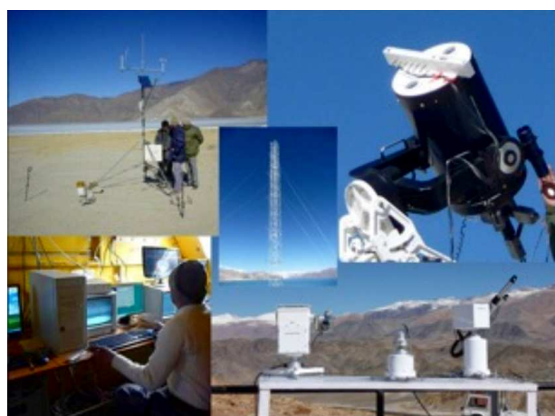
Fig. 4: Collage of instruments, clock wise from top right, (1) SDIMM and SHABAR, (2) sky radiometer and all sky camera, (3) data acquisition facility at Merak site of Pangong lake, and (4) AWS at Merak. The picture in the middle is of the micro thermal tower at Merak
