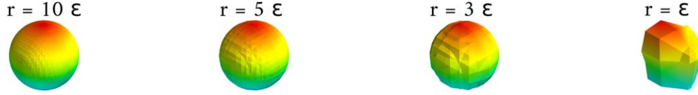
Figure 12. We exhibit the breakdown in accuracy of the marching tetrahedron algorithm. After generating a smooth spherical density field \delta(x, y, z) = \delta(r) as in Equation (55), we construct a surface of constant density around the central point. We decrease the radius of the sphere: from left to right, the radius is r = 10, 5, 3, 1 \times \epsilon , where \epsilon is the resolution of the grid.
