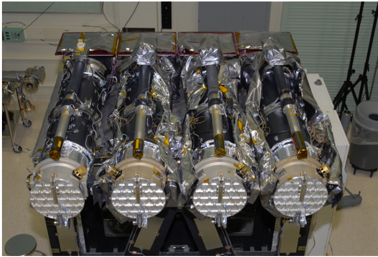
FIGURE 2.2: The array of four AIA telescopes mounted on the SDO spacecraft. Credit: Lemen et al. (2012a)
