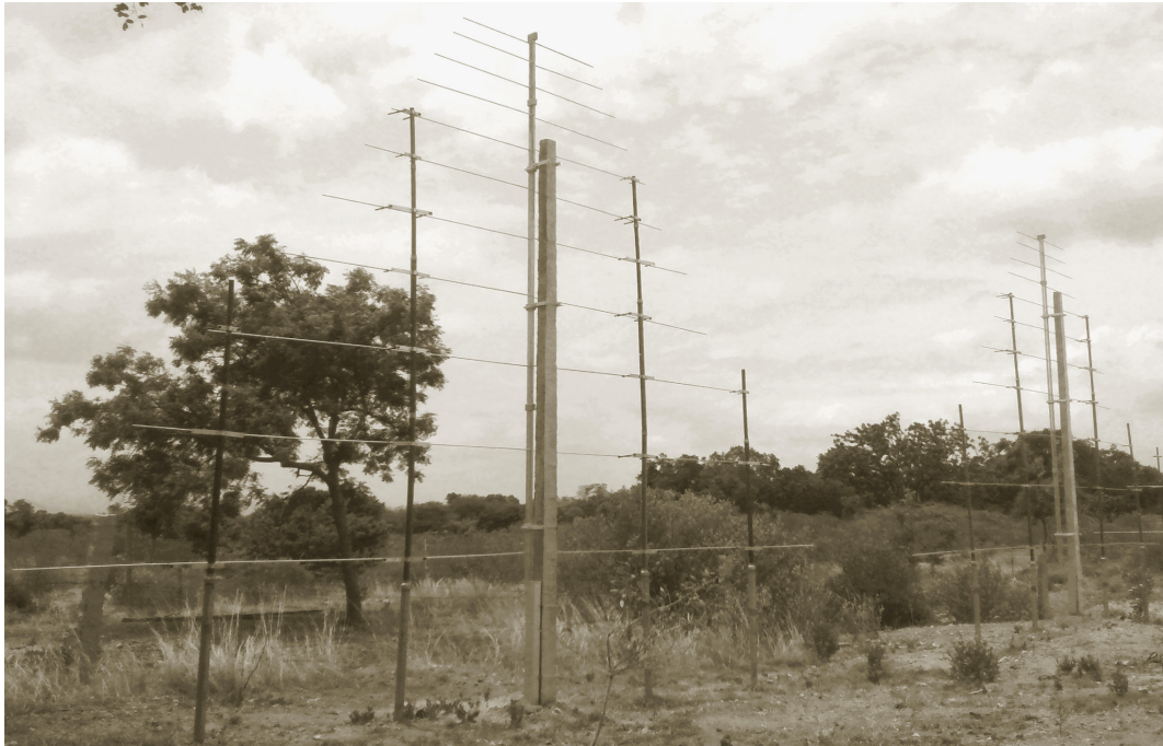
Figure 4.1: A view of the two LPDAs used in the spectrograph.
