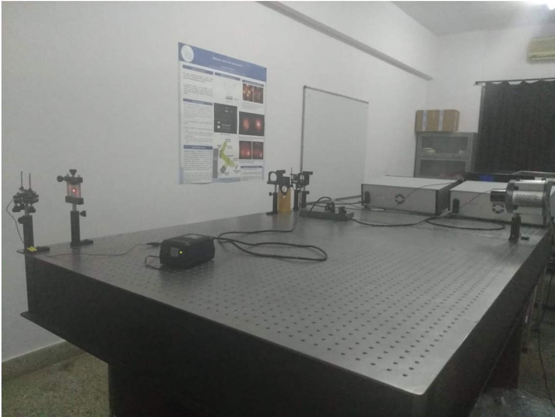
FIGURE 3.2: Setup used in lab to calibrate response of actuator
