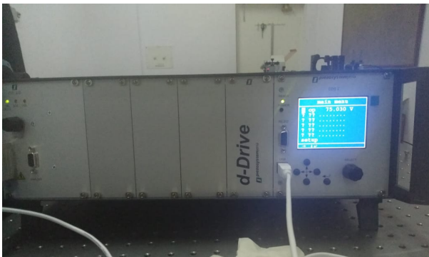
FIGURE F.1: Amplifier evd300-it amplifies the signal sent from the computer before applying it to the actuator
