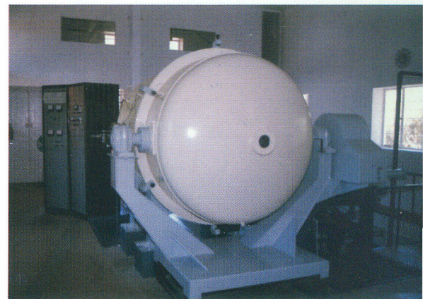
1.6m vacuum coating plant in VBO
