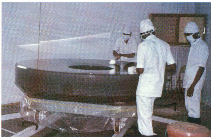
The 234-cm mirror being cleaned for aluminizing in the 2.8-mvacuum coating plant in Kavalur.
