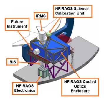
**Figure 1.** Schematic diagram of the NFIRAOS.
