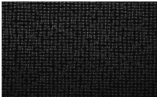
Figure 4. A sample spot pattern image captured by the SHWS camera with the phase plate in the beam path
